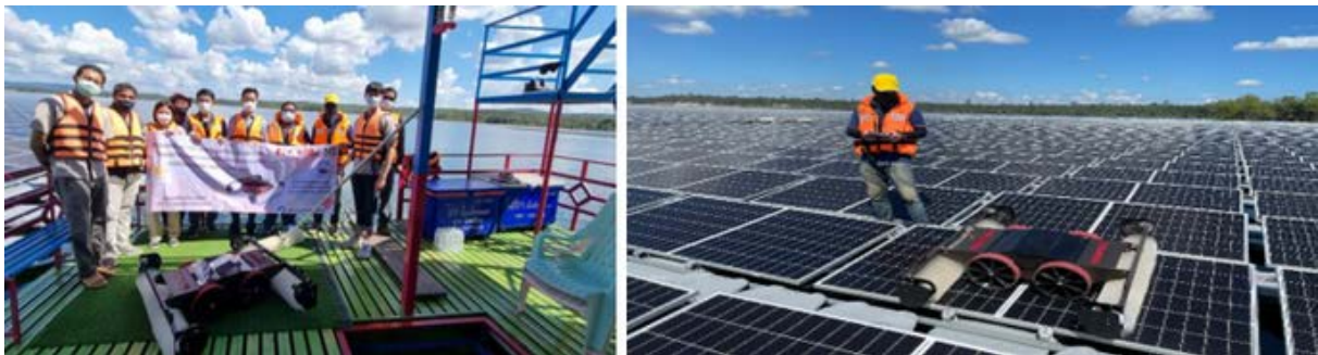
Cleaning Robot for Floating Solar Panels
